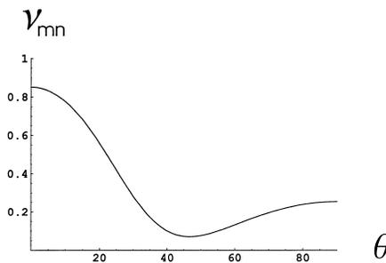
Figure 2. Variation of the Poisson ratio  $\nu_{mn}$  in the direction  $\mathbf{m}$  due to stress in the orthogonal direction  $\mathbf{n}$ . Both directions are in the plane containing the axis of transverse isotropy of a zinc crystal.
