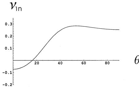
Figure 1. Variation of the Poisson ratio  $\nu_{1n}$  in the direction 1 due to stress in the direction  $\mathbf{n}$ , at an angle  $\theta$  from the basal plane of a zinc crystal. The axis 1 is normal to the plane containing the axis of transverse isotropy and the direction  $\mathbf{n}$ .
