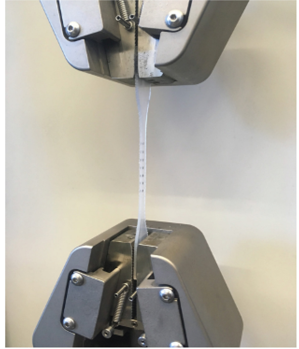
Fig. 4 – Uniaxial tensile testing of ethylene vinyl acetate tube material [MTS-Criterion tester]. The initial length of the specimen is l_0 = 140 mm, and the initial dimensions of the rectangular cross section are 3 mm × 1.59 mm.
