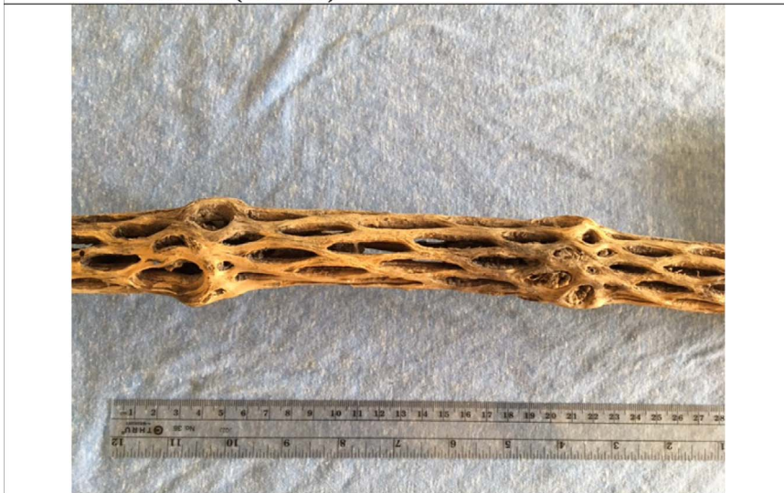
Lightweight structures that have fascinated Prof. Meyers and have inspired his studies in biological materials: (a) toucan beak with cellular core covered by keratin shell; (b) Hollow Cholla cactus trunk consisting of weaved wood fibers. Both structures maximize the stiffness/weight ratio.
