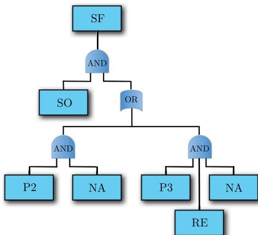
Fig. 1. The fault tree used in [26] to assess the probability of failure of a permeable reactive barrier to remediate a contaminant plume.
