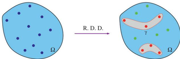
**Fig. 3.** A schematic representation of a subsurface environment  $\Omega$ , whose property is sampled at the locations indicated by dots. Random domain decompositions (RDDs) [184,185] can be used to delineate probabilistically the boundaries  $\gamma$  of highly permeable sub-domains and to quantify predictive uncertainty associated with such delineation.
