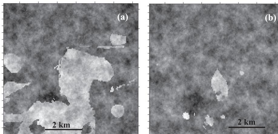
**Fig. 4.** A probabilistic reconstruction of the high-conductivity (light shades) and low-conductivity (dark shades) heterogeneous lithofacies in an aquitard [75]. Figures (a) and (b) display reconstructions with probability 74% and 87%, respectively.
