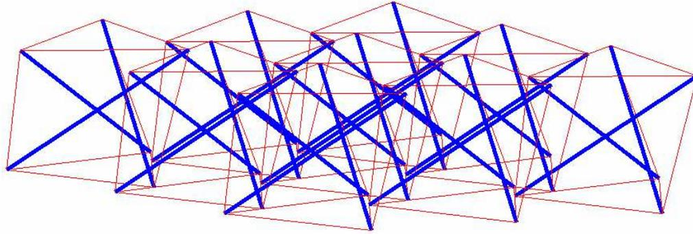
**Figure 2.** A 9 Stable 3-Bar Units Tensegrity Plate
