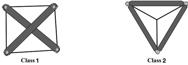
FIGURE 18.4 Class 1 and Class 2 tense-grity structures.
