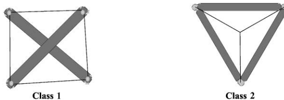
Fig. 4. Class 1 and Class 2 tensegrity structures.
