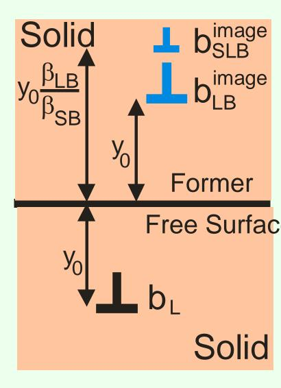
$$\{u_x\}_L = \frac{b_L}{2\pi} \tan^{-1} \frac{\beta_L (y + y_0)}{x}, \qquad \{u_y\}_L = \frac{b_L \beta_L}{2\pi} \ln \sqrt{x^2 + \beta_L^2 (y + y_0)^2},$$
