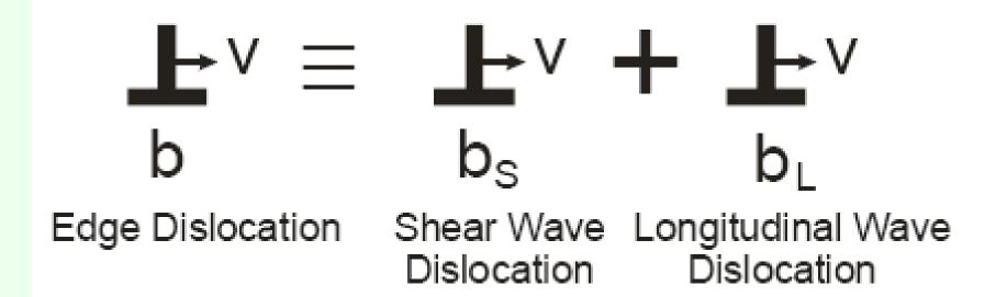
Figure 3. Moving edge dislocation considered to be sum of moving edge shear wave dislocation component and moving edge longitudinal wave dislocation component.
