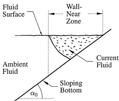
Fig. 2. Sketch of cross-section of local flow geometry in wall-near zone in the case of currents propagating along an inclined boundary
