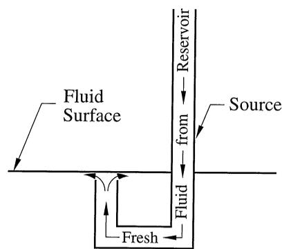
Fig. 3. Sketch of cross-section of flow geometry near the source illustrating the direction of the fluid discharge
