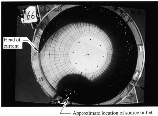
Fig. 4. Flow visualization taken from a video recording of an experiment with  $\Omega = 0.5 \text{ rad s}^{-1}$ ,  $g' = 86.3 \text{ cm s}^{-2}$  and  $q_0 = 20 \text{ cm}^3 \text{ s}^{-1}$  ( $\Pi = 0.063$ ) at  $t \approx 60 \text{ s}$ . The current flows along a vertical wall. The sense of the rotation of the turntable is anti-clockwise. The current also propagates anti-clockwise such that it moves along the wall of the tank keeping the wall (coast) to its right
