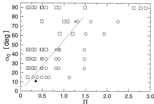
Fig. 6. Experimental data points showing for which inclination angles  $\alpha_0$  attached heads ( $\square$ ), detached heads ( $\circ$ ), and double heads ( $\times$ ), were observed for different numeric values of the non-dimensional parameter  $\Pi$ ,  $\blacktriangle$ : data point obtained from Whitehead and Chapman (1986), .....  $\alpha_0 = 55 \cdot \Pi$
