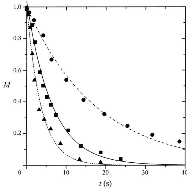
FIGURE 8. Non-dimensional salt-water mass  $M(t)$  for some experiments performed using a single grid as porous surface. The symbols correspond to:  $x_0 \approx 15$  cm and  $g' = 9.8$  cm s $^{-2}$  (●), 49 cm s $^{-2}$  (■), and 98 cm s $^{-2}$  (▲). The best-fit exponential functions have decay times  $\tau = 17.57$ , 6.53 s and 3.52 s, respectively.
