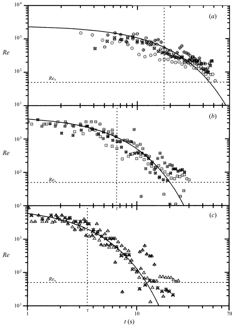
FIGURE 5. Log-log variation of  $Re$  with time for: (a)  $g' = 9.8 \text{ cm s}^{-2}$ , (b)  $g' = 49 \text{ cm s}^{-2}$ , and (c)  $g' = 98 \text{ cm s}^{-2}$ , when the porous substrate is a single grid. The evolution of  $Re$  described by the solid lines is given by (4.9) for the corresponding parameters.
