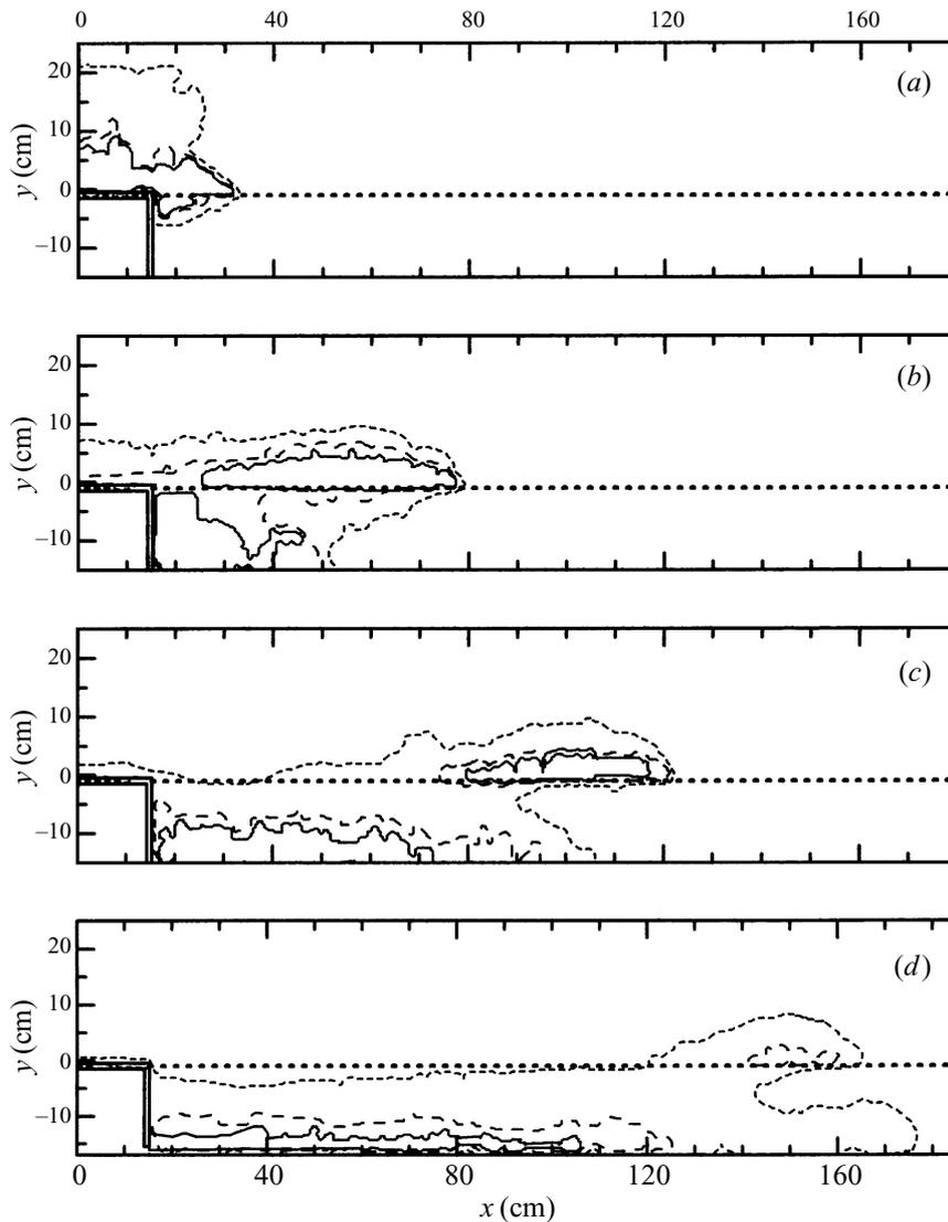
FIGURE 6. Evolution of the iso-density contours obtained for the experiment with  $x_0 = 15.2$  cm and  $g' = 50.47$  cm s $^{-2}$  at (a)  $t = 1.24$ , (b) 5.08, (c) 10.36, (d) 18.70 s for which  $Re = 3800$ , 1500, 400 and 60, respectively.
