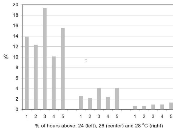
**Figure 11** Percentage of hours above 24, 26 and 28°C during office operation hours (8 am–6 pm)
