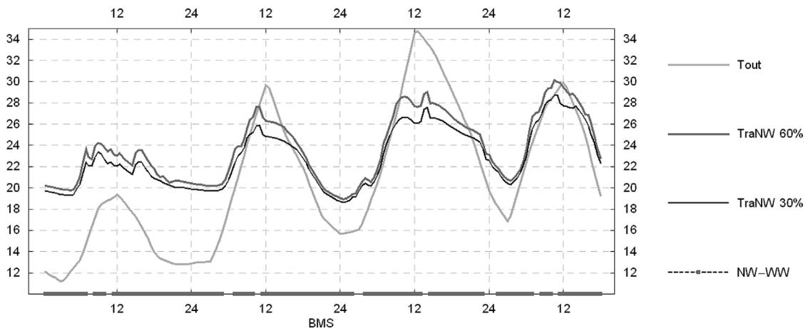
**Figure 9** Effects of scrim transmissivity on the comfort temperature in the SE bay for a sequence of warm days in July
