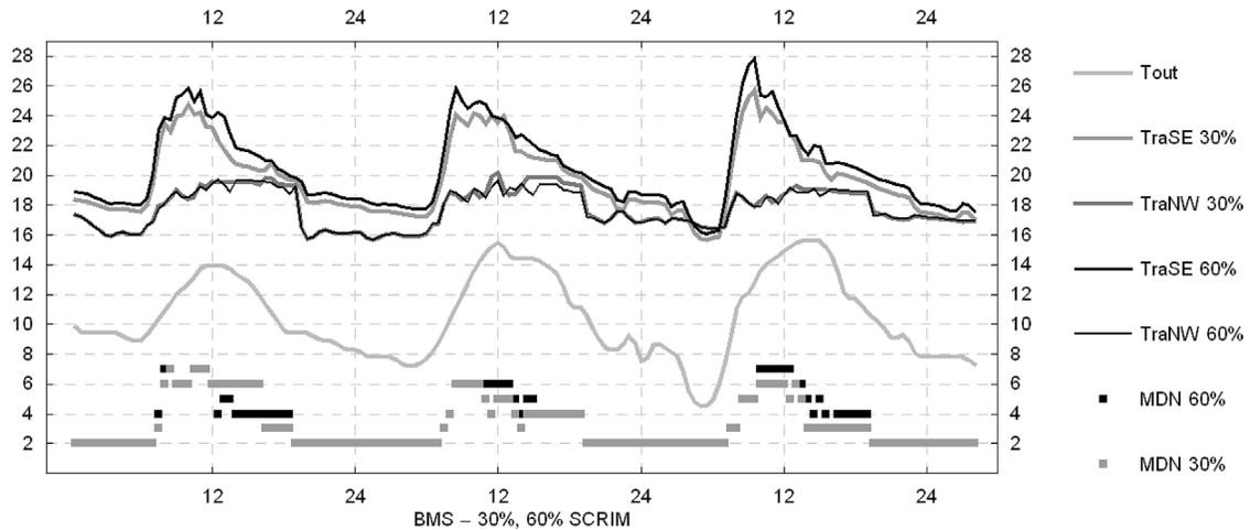
**Figure 10** Effects of scrim transmissivity on the temperature in both bays during cold days
