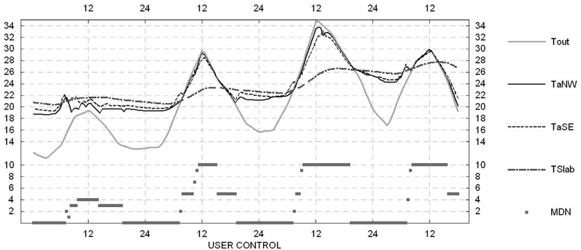
**Figure 7** Indoor temperatures for a building with no BMS and uninformed users (case 5). In this chart, MDN is the user operable opening level, from closed (0) to fully open (10).
