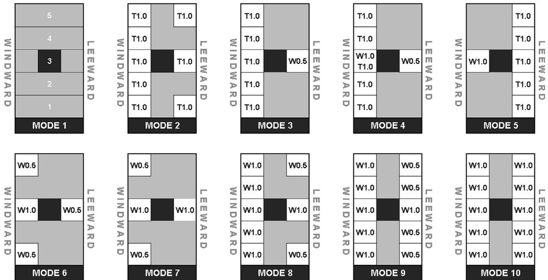
**Figure 3** Schematic representation of the aperture modes. Each floor of the building is divided into two symmetrical sides. The figure shows one half of one floor. The black square in the center of the figures is an elevator/service core that creates an obstruction to cross-ventilation airflow
