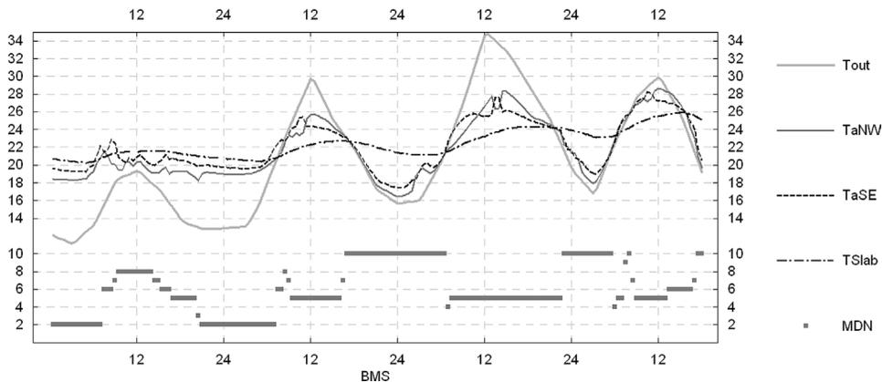
**Figure 5** Predicted temperatures for case 1 in a sequence of warm days in July. All temperatures in °C.  $T_{out}$ : outside air temperature.  $T_{aNW}$ : average air temperature in the North West bay.  $T_{aSE}$ : average air temperature in the South East bay.  $T_{slab}$ : average surface temperature of the concrete ceiling slab. MDN: BMS system window opening mode
