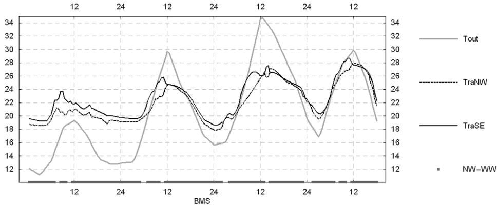
**Figure 6** Predicted comfort temperature and airflow direction for a sequence of warm days (case 1). All temperatures in °C. The two bay temperatures shown (Tra-NW, SE) are obtained by calculating the average between the average air and mean radiation temperature in each zone. The grey squares labeled NW–WW signal cross-ventilation airflow entering the building in the NW bay and exiting in the SE bay
