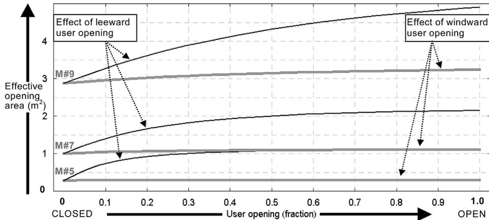
**Figure 4** Variation of effective opening area ( $A^*$ , expression (1)) with user opening. The three pairs of lines (from bottom to top) show the effective area for, respectively, opening MDN 5, 7 and 9. The grey lines are obtained by varying the user operable opening area on the windward side. The black lines are obtained by varying the user operable opening area on the leeward side
