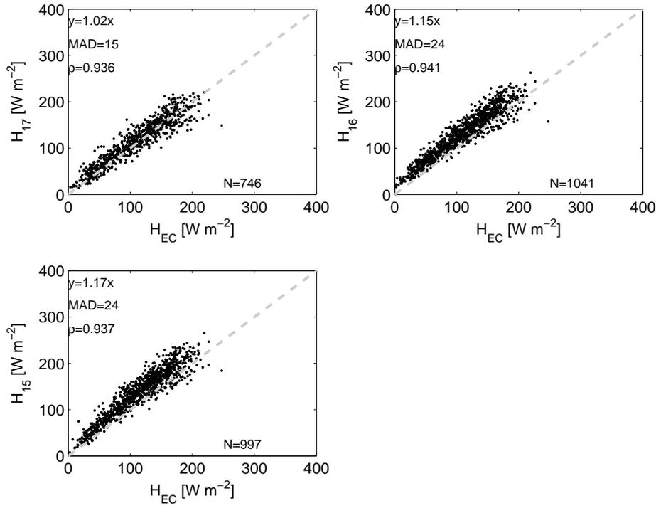
**Fig. 7** Scatter plots of sensible heat flux measurements from eddy-correlation ( $H_{EC}$ ) versus different LASs (only the last two digits of the serial number are shown in the axis label) for experiment S3. The figure also shows the linear fit, mean absolute deviation (MAD in  $\text{W m}^{-2}$ ), correlation coefficient  $\rho$ , and number of samples  $N$ .
