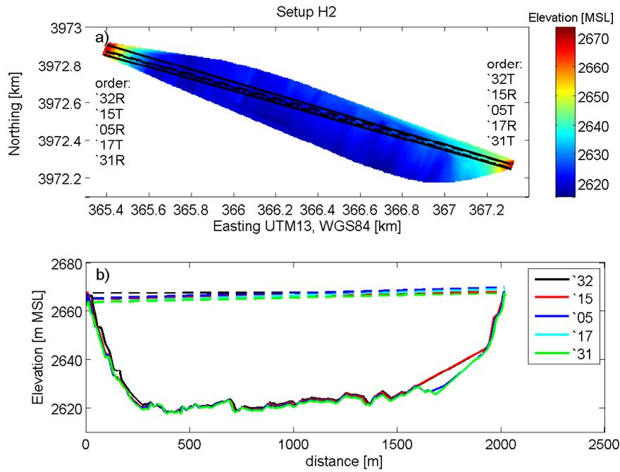
**Fig. 2** a) Bird's eye view of the digital elevation model (DEM) of the VCNP experiment H2 with LAS transects. The legend gives the last two digits of the LAS serial number (Table 1). The EC tower coordinates are 366.7 E and 3971.1 N (UTM13, WGS84). Receivers and transmitters were alternated at each site. (b) Profile of transects.
