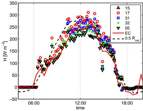
**Fig. 4** Example time series of the net radiation ( $R_{\text{net}}$  rescaled by  $1/2$ ) and sensible heat flux  $H$  from LAS and EC for experiment H1 on June 19, 2006.
