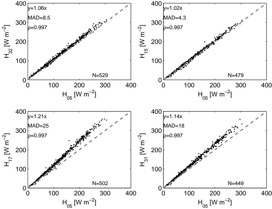
**Fig. 5** Scatter plots of sensible heat flux measurements from serial number  $^{0300}05$  ( $x$ -axis) vs the other LASs (only the last two digits of the serial number are shown in the axis labels) for experiment H1. The text indicates the linear fit, mean absolute deviation (MAD in  $\text{W m}^{-2}$ ), correlation coefficient  $\rho$ , and number of samples  $N$ . The grey dashed line is the 1:1 line.
