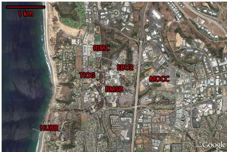
Figure 1: Map of the UCSD solar resource sites, showing proximity to the Pacific Ocean (left), and Interstate 5 (center). From EBU2, distances and headings are: BMSB(0.69km, 205°), HUBB (2.47km, 230°), MOCC (0.95km, 105°), RIMC (0.80km, 300°), and TIOG (1.00km, 255°). Map © 2010 Google – Image © 2010 TerraMetrics.
