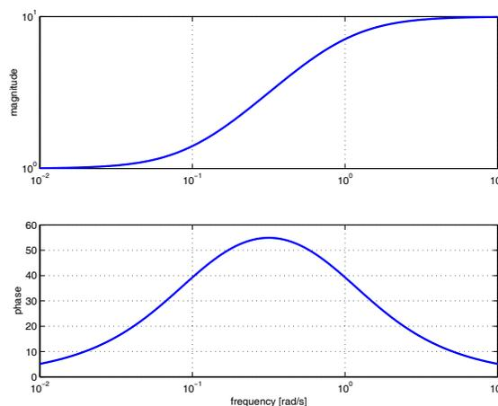
Bode plot for lead/lag compensator with parameters
