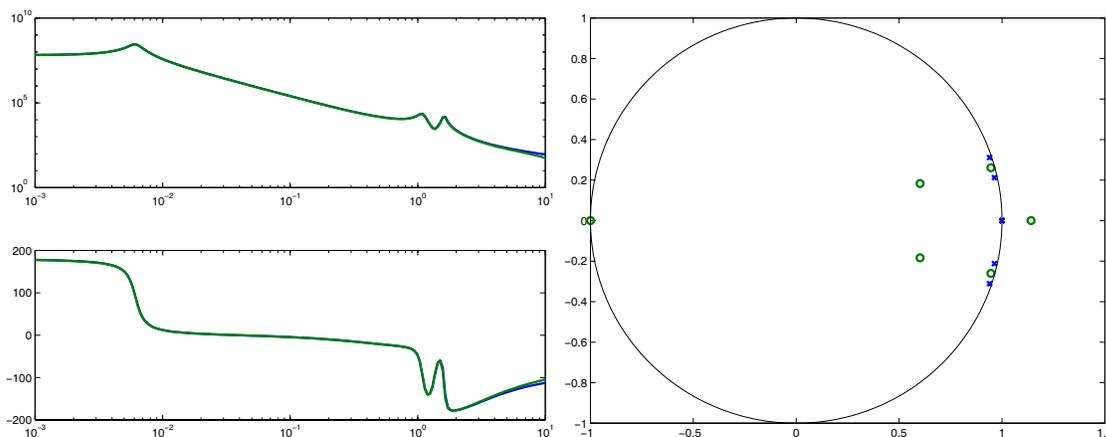
Bode plot of continuous and discrete time model (left) and pole/zero plot of discrete time model (right)
