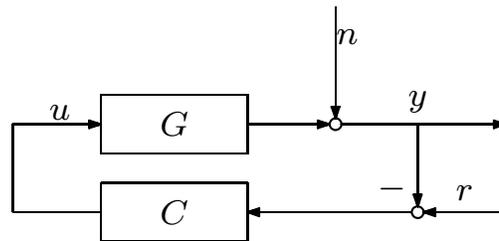
Loopgain  $L$  is series connection of model  $G$  and controller  $C$ :
