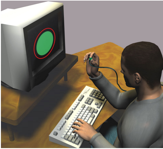
Fig. 3. Experimental setup. The subject sits in front of a monitor, holding a 3D absolute position sensor (Polhemus Liberty). Here n_h = 2 , n_s = 1 . The center-stationary green circle is the target, whose diameter ( s(t) ) fluctuates according to damped Brownian motion, and there is a concentric 'cursor' (red circle) whose diameter is z(t) = m(t)^T h(t) , with m(t) fluctuating according to an independent damped Brownian motion. The subject is then told to move however possible to try to keep z(t) = s(t) . Trials are 1 min., started by a key-press and sampling rate is 50Hz.
