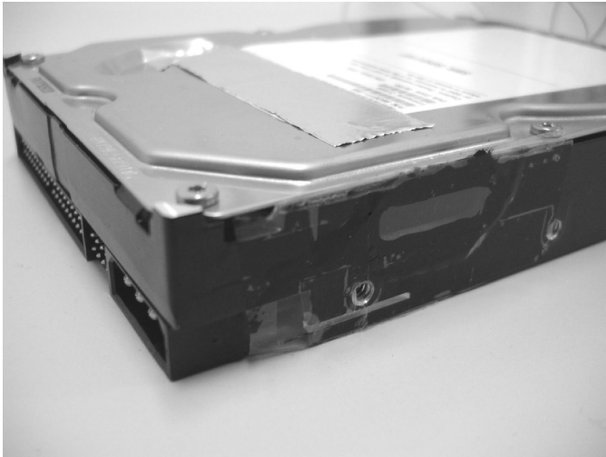
Fig. 1. Modified hard disk drive used in the experiment. A lateral opening has been made on the case in order to let the read/write head accessible to the reference laser beam of the LDV. A transparent glass slide applied on the hole protects the drive against dust.
