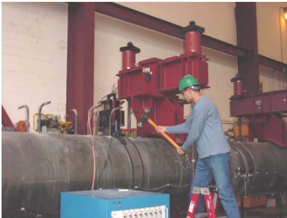
Figure 8. Impact hammer test on the girder
