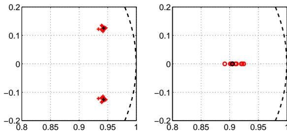
Fig. 4. Pole (left figure) and zero (right figure) locations of the identified linear dynamical system. The black cross and circle indicate the real linear dynamical system. The colored crosses and circles indicate estimated linear dynamical systems. The SNR of each data set is greater than 50dB.
