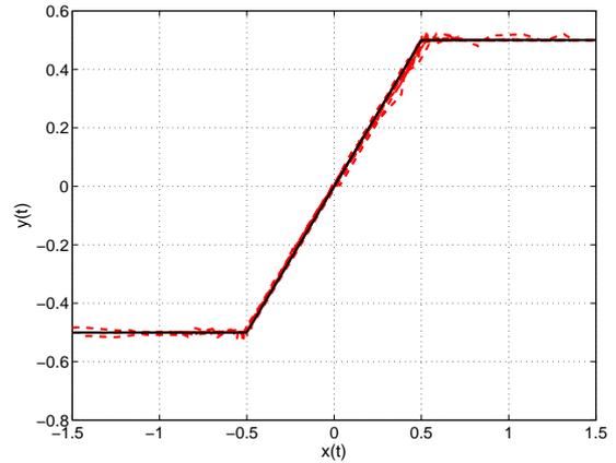
Fig. 5. The plot of the identified static nonlinear function. The black solid line indicates the real static nonlinear function. The (colored) dashed lines indicate estimated static nonlinear functions by using twenty different sets of data. The SNR of each data set is greater than 50dB.
