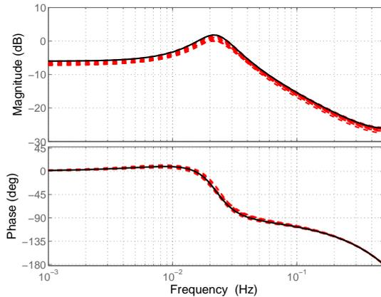
Fig. 3. The Bode plot of the identified linear dynamical system. The black solid line indicates the real linear dynamical system. The (colored) dashed lines indicate estimated linear dynamical systems by using twenty different sets of data. The SNR of each data set is greater than 50dB.
