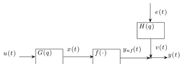
Fig. 1. Wiener system with output noise.
