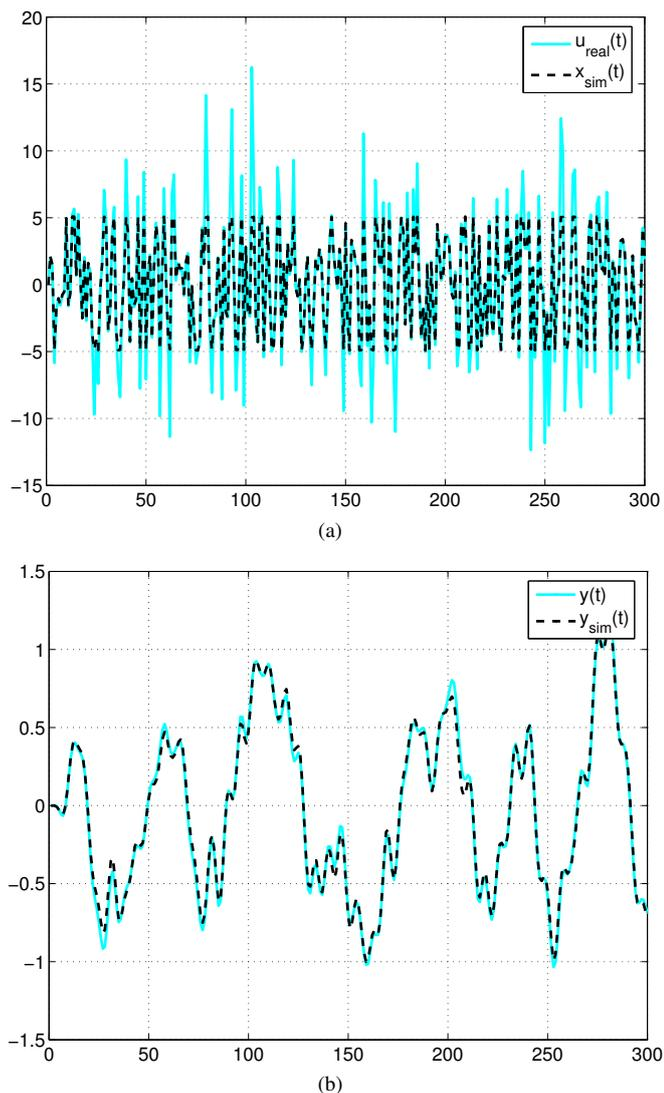
Fig. 6. (a) The plot of the measured input signal  $u(t)$  and the simulated intermediate signal  $x_{sim}(t)$ . The  $\pm 5V$  input saturation is very nicely estimated. (b) The plot of the measured output signal  $y(t)$  and the simulated output signal  $y_{sim}(t)$ .
