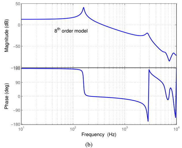
Fig. 5. (a) The plot of the identified static nonlinearity function  $\hat{f}(\cdot)$ . (b) The Bode plot of the identified linear dynamic system  $\hat{G}(q)$ .
