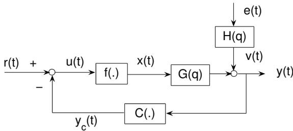
Fig. 1. closed-loop Hammerstein system.
