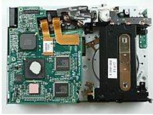
Fig. 3. Quantum LTO-3 tape drive.
