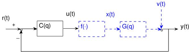
Fig. 4. Closed-loop experimental setup of a Quantum LTO-3 tape drive. The excitation signal  $r(t)$  and the linear controller  $C(q)$  are known. The input to the static nonlinearity  $u(t)$  and the output  $y(t)$  are measured. The static nonlinearity  $f(\cdot)$  and linear dynamic system  $G(q)$  are unknown and need to be estimated under a unknown colored disturbance  $v(t)$  (the dotted line indicates unknown parts and the solid line indicates the known parts).
