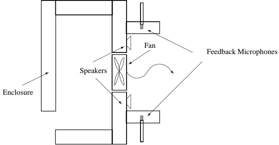
Figure 3. Active noise canceling system used to eliminate the unwanted noise from a cooling fan.
