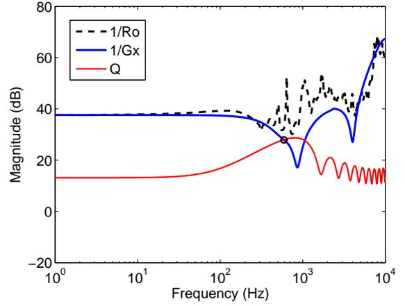
Figure 10. Controller enhancement filter  $Q$  for a frequency of 592 Hz.
