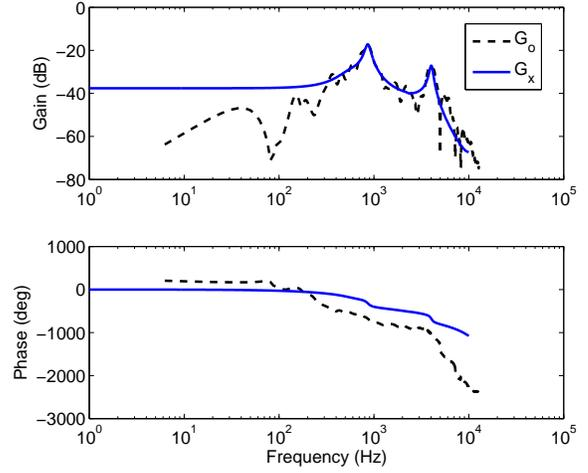
Figure 7. Frequency response of model  $G_x$  and the true system  $G_o$ .
