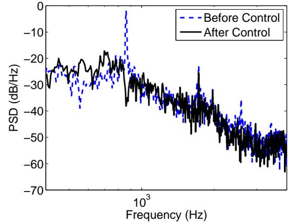
Figure 11. Power spectral density of the acoustic noise generated by the cooling fan before and after feedback control.
