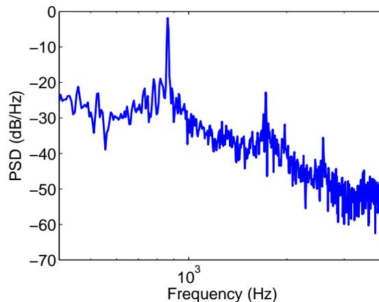
Figure 2. Power spectral density of the acoustic noise generated by the cooling fan.
