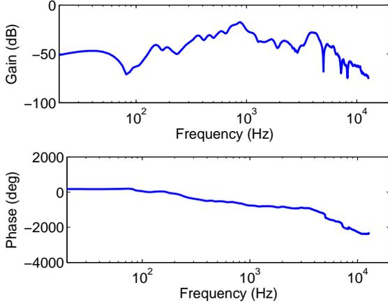
Figure 6. Frequency response between the feedback microphone and speaker.
