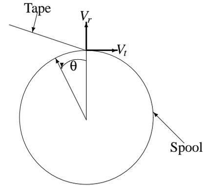
Figure 1. Spool with constant tape speed.
