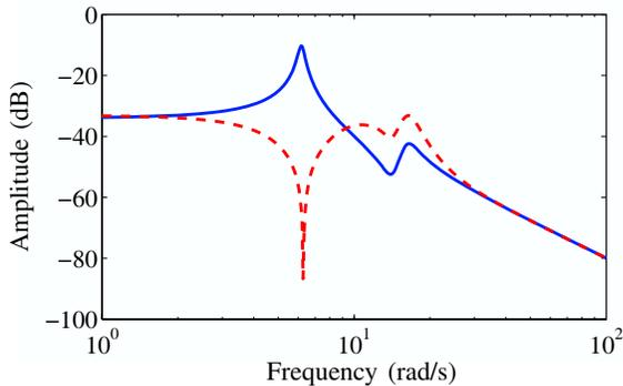
Fig. 4. Singular value plot of  $T_{yd}(s)$  (Solid) and the closed loop system with the non-scheduled controller (Dashed).
