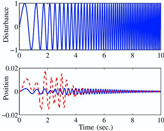
Fig. 3. Top: Disturbance signal  $d(t)$ . Bottom: Closed loop system with scheduled IMB control (Solid) and closed loop system with non-scheduled IMB control (Dashed).
