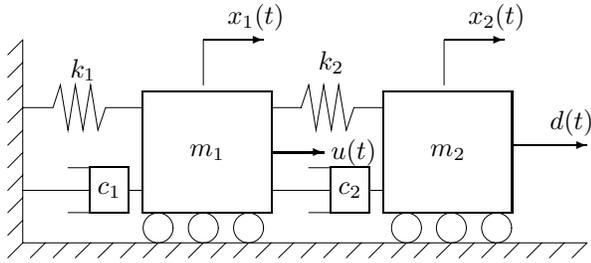
Fig. 2. Simple mass-spring-damper system.
