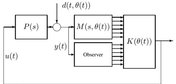
Fig. 1. Scheduled internal model-based controller connected in feedback to the plant  $P(s)$ .
