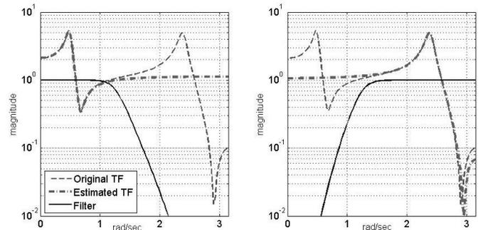
**Fig.1** Estimation of a 4<sup>th</sup> order system by a 2<sup>nd</sup> order model
