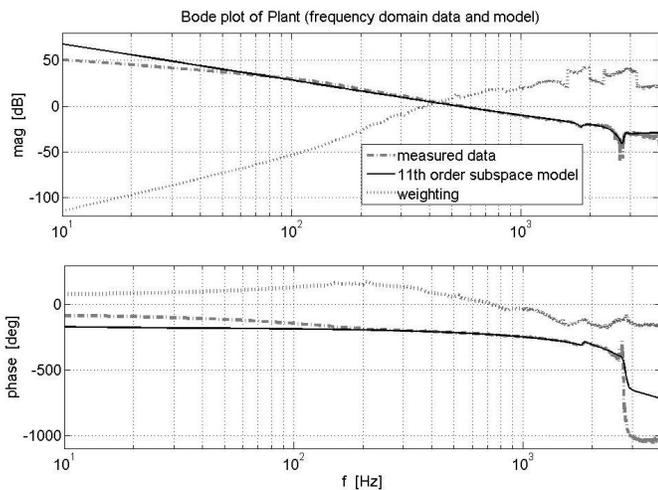
**Fig.3** 11<sup>th</sup> order subspace model of the plant
