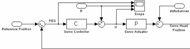
**Fig.2** Schematic of the servo system and relevant signals
