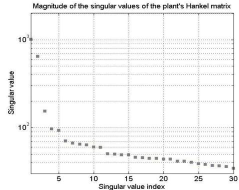
**Fig.5** Magnitude of the singular values of the plant Hankel matrix
