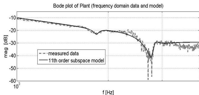
**Fig.4** High frequency response of the plant
