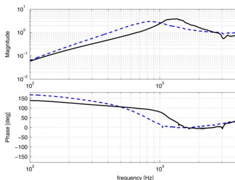
Fig. 3. Measured disk drive sensitivity functions resulting from servo controllers PID (dashed-line) and reduced-order Hoc (solid-line). (Color version available online at <http://ieeexplore.ieee.org>.)
