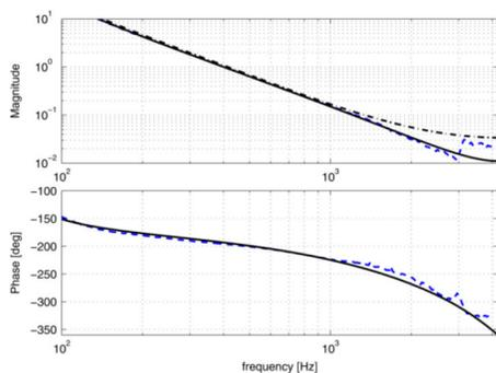
Fig. 1. Frequency response of the measured plant (dashed-line) and a nominal model (solid-line) with additive uncertainty (dash-dotted-line). (Color version available online at <http://ieeexplore.ieee.org>.)
