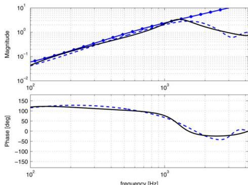
Fig. 2. Performance weight (solid-circles-line) and the sensitivity functions resulting from full-order  $\mathcal{H}_\infty$  control synthesis (dashed-line) and reduced-order controller (solid-line). (Color version available online at <http://ieeexplore.ieee.org>.)
