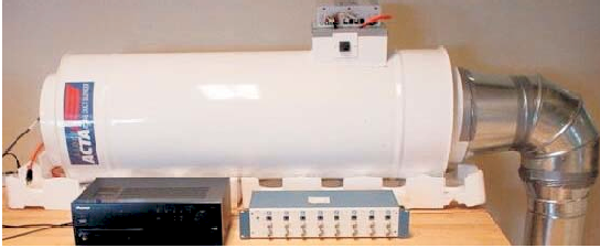
Figure 3. ACTA AIRDUCT SILENCER LOCATED IN THE SYSTEM IDENTIFICATION AND CONTROL LABORATORY AT UCSD
