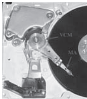
Fig. 1. Dual-Stage Suspension Disk Drive with Hutchinson Magnum 5E PZT dual-stage actuator
