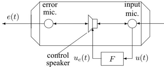
Fig. 2. Schematics of ANC system
