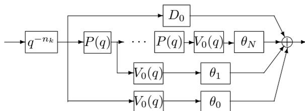
Fig. 4. Basic structure of generalized FIR filter
