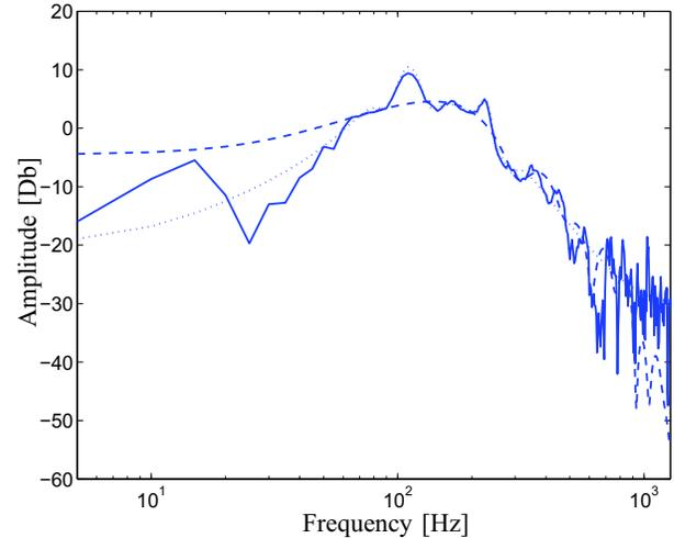
Fig. 5. Spectral analysis of ideal feedforward controller (solid), approximation using FIR filter estimation (dashed) and approximation using generalized FIR filter estimation (dotted)
