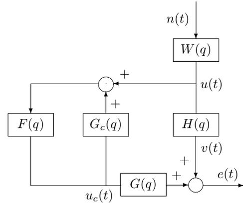
Fig. 3. Block diagram of ANC system with feedforward
