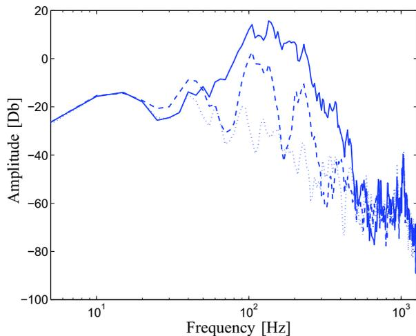
Fig. 6. Estimate of spectral contents of error microphone signal  $e(t)$  without ANC (solid), with ANC using 20th order FIR filter (dashed) and with ANC using 20th order generalized FIR filter (dotted)
