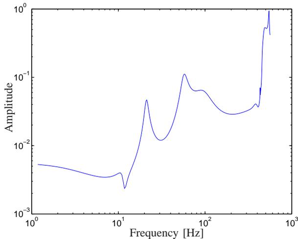
Fig. 6. Robust stability test for multiplicative uncertainty model  $\mathcal{P}_m$
