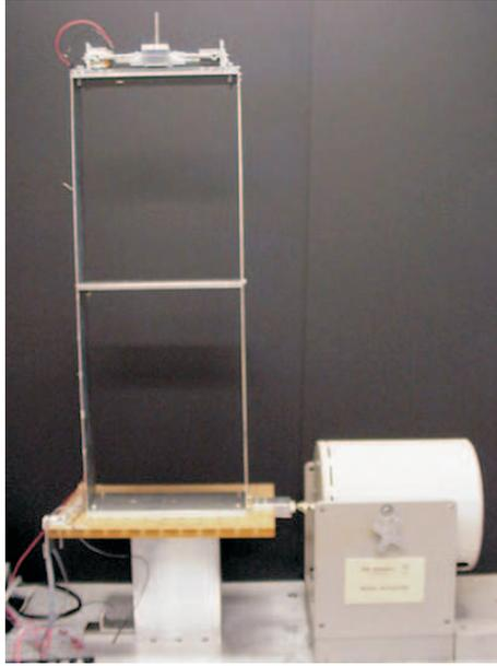
Fig. 1. Flexible test structure used for model validation comparison
