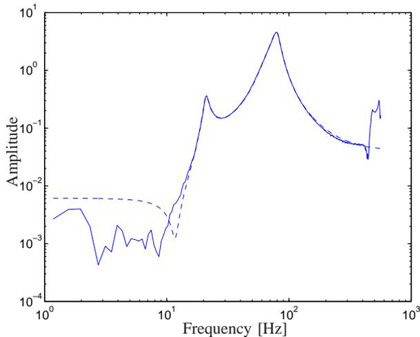
Fig. 2. Amplitude Bode plot of open-loop frequency domain data (solid) and 6th order nominal open-loop model (dashed)
