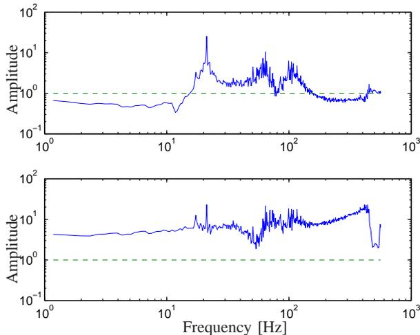
Fig. 7. Model Validation Test, multiplicative uncertainty description (top) and coprime factor uncertainty description (bottom)
