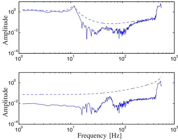
Fig. 5. Amplitude bode plot (solid) of perturbation and parametric upper bound (dashed)  $\Delta_m$  (top) and  $\Delta_{cf}$  (bottom)
