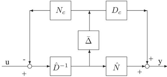
Fig. 4. Uncertainty Model Based on Perturbations on Coprime Factorizations
