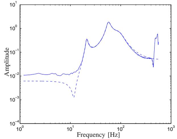
Fig. 3. Amplitude bode plot of closed-loop frequency domain data (solid) and nominal closed-loop model  $\frac{\hat{P}}{1+C\hat{P}}$  (dashed)
