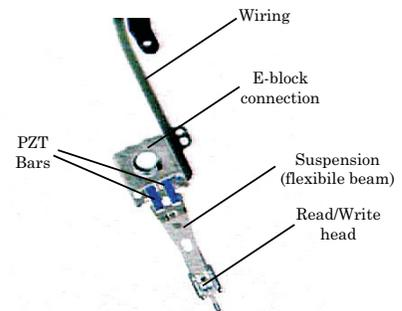
is a 8<sup>th</sup> order transfer function, composed of a VCM mode at 25Hz, an E-block mode at 5kHz, a suspension torsion mode at 5.9kHz and a suspension sway mode at 9kHz.  $P_{ma}$  is a 4<sup>th</sup> order
