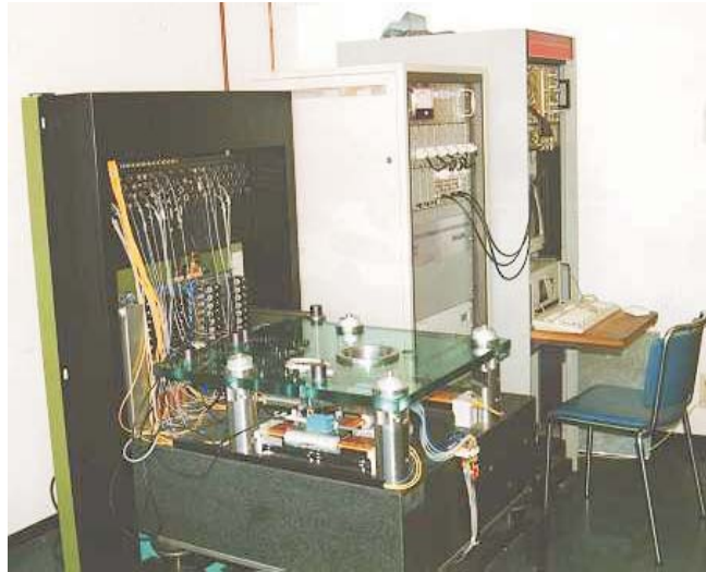
Fig. 8.2: Experimental set up with (from left to right) the wafer stage, interface and host computer with digital signal processor.
