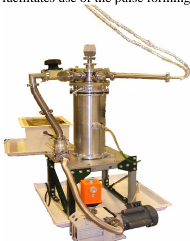
FIGURE 1. A photograph of an x-pinch pulser. A compact Marx bank may be seen in the background.
