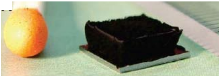
Figure 5. SWNT forest grown with water-assisted CVD which shows 2.5-mm tall SWNT forest on a 7 mm X 7 mm silicon chip. A matchstick is shown on the left for size reference. From Reference [63]. Reprinted with permission from AAAS.
