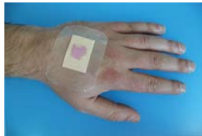
▲ EMFT scientists developed a dressing that changes color from yellow to purple if the pH of the skin is between 6.5 and 8.5 — a range that frequently indicates infection. Photo courtesy of Fraunhofer EMFT.
