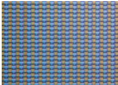
▲ Using a new templated-growth technique, Georgia Tech researchers have fabricated an array of 10,000 graphene transistors. The graphene’s smooth edges help to avoid electron scattering. Photo courtesy of Walt de Heer.
