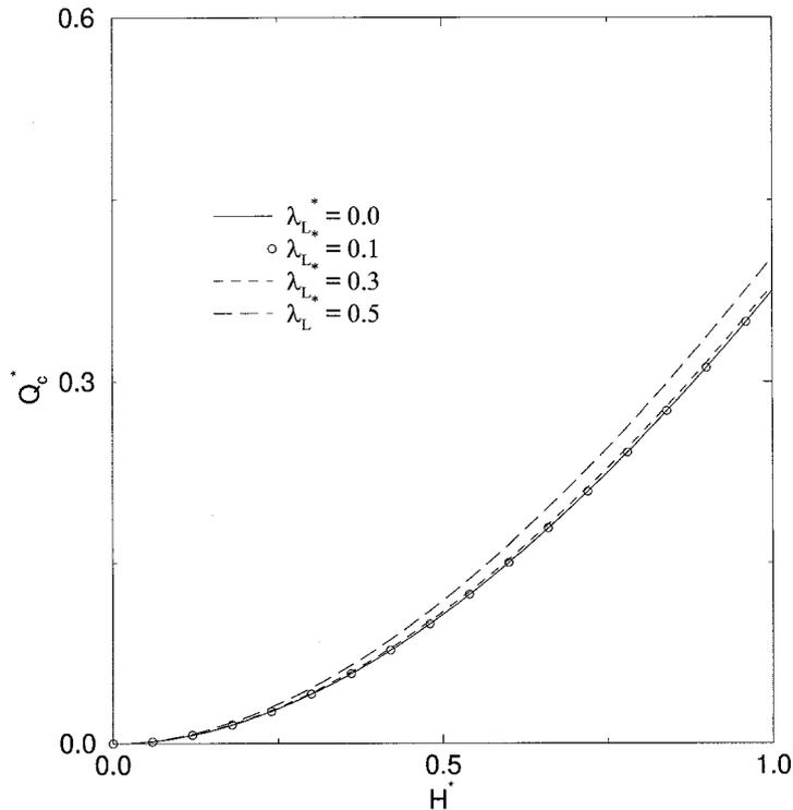
Figure 2(b). Dimensionless contaminant flux,  $Q_c^*$ , through trapezoidal embankment ( $m = 1$ ) as a function of dimensionless upstream head,  $H^*$ , for  $h_0^* = 0$  and different values of  $\lambda_{L^*}$ .
