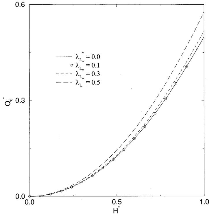
Figure 2(a). Dimensionless contaminant flux,  $Q_c^*$ , through rectangular embankment ( $m = 0$ ) as a function of dimensionless upstream head,  $H^*$ , for  $h_0^* = 0$  and different values of  $\lambda_{L^*}$ .
