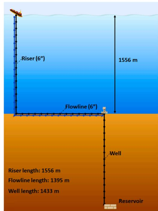
Fig. 2. Schematic of a simplified production well implemented in the flow simulator.
