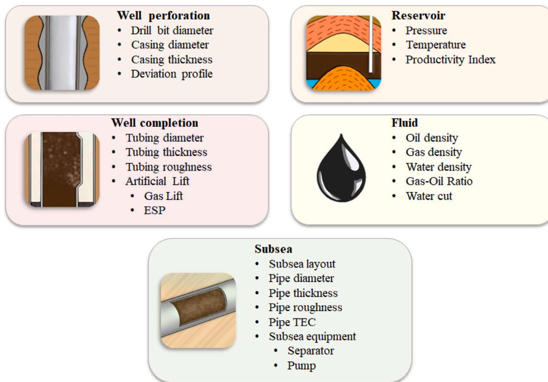
Fig. 1. Physical properties that provide input for a steady-state black-oil flow simulation.
