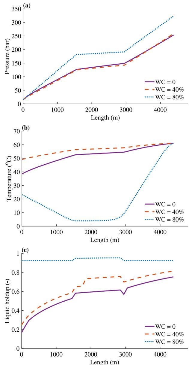
Fig. A.1. (a) Pressure, (b) temperature, and (c) liquid holdup behaviors at the steady-state regime in the wellbore and production line for watercut values of 0%, 40%, and 80%, representing the beginning, middle and end of the production lifetime, respectively.
